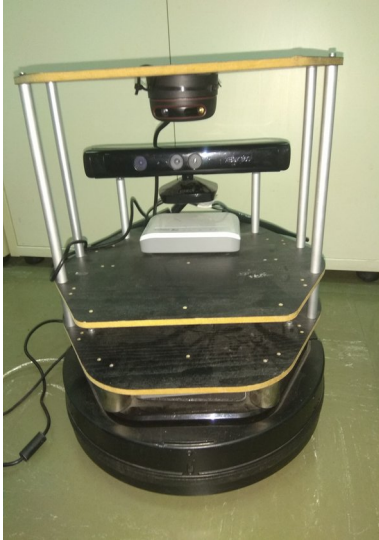
Figure 36: RPLIDAR is mounted on the top plate of Turtlebot, Kinect is located under Rplidar.
