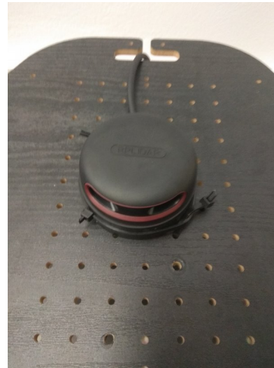
Figure 39: Close view of RPLidar mounted on top of the top plate of Turtlebot
