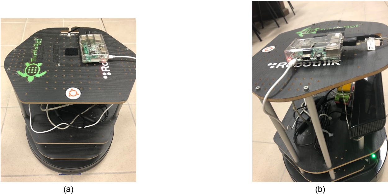
Figure 4.6: The Turtlebot UGV with XBOX Kinect and Raspberry Pi computing modules.
